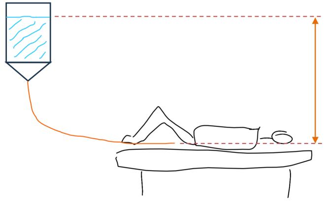
Outlet pressure depends ONLY on this height, between top of water and end of outlet tube
